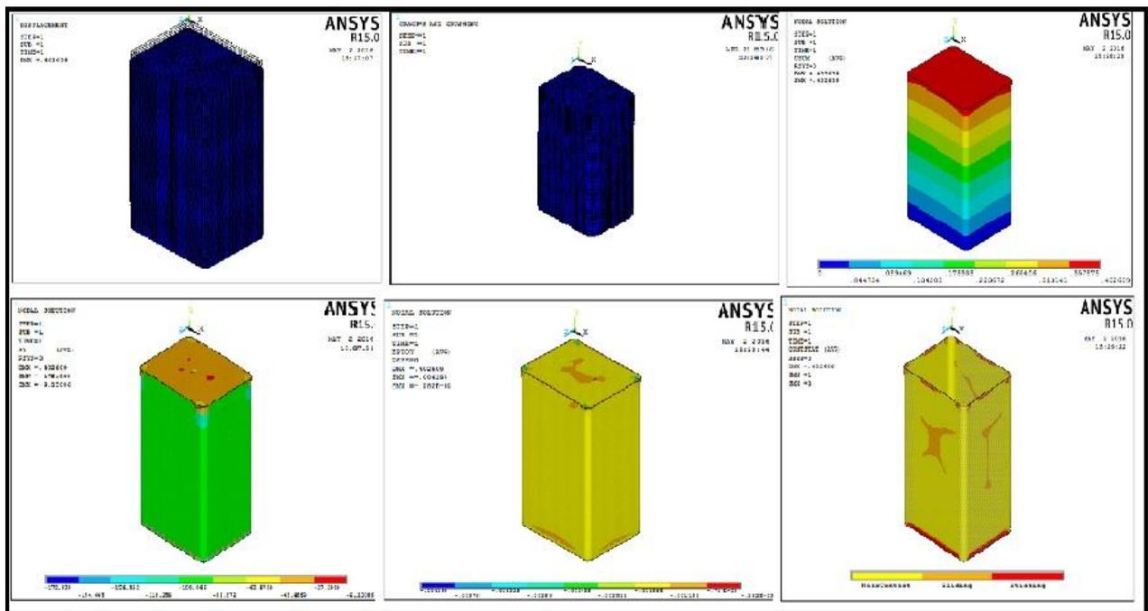
Fig 6 Deformation, stress, strain and contact status
